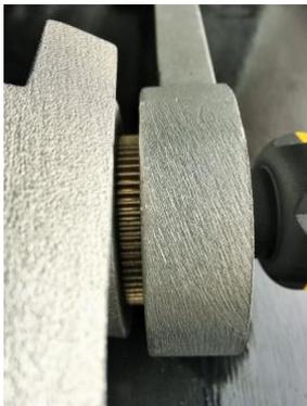
Gear threads between the stabilising leg and clamp.
