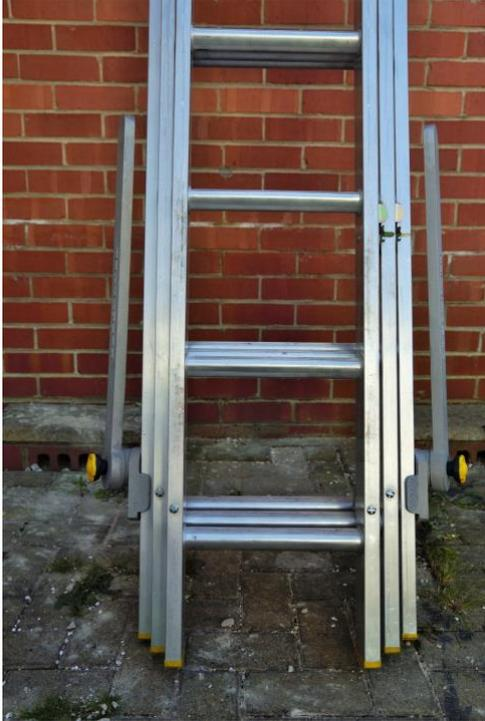
2. To use the legs loosen the yellow plastic knob, pull the stabilising leg out and twist it down to the required position. Push the leg inwards and make sure the interlocking gears have locked into place then tighten the knob. **If you can see the gear threads it means the leg is not locked into place.**
