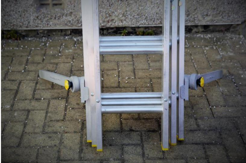
5. Place device into storage position once ladder is not required. Please **do not** rest the ladder on the yellow plastic knobs.
